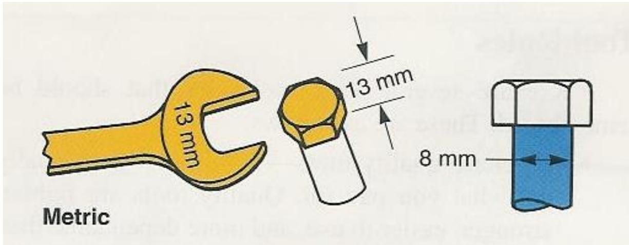
**Metric** wrench sizes are given in **millimeters**. The measurement is the wide of the jaw opening. The wrench size is not the same as the bolt size.
